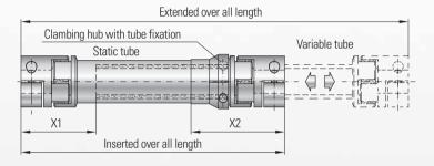
The extended over all length and the inserted over all length are related. Depending on the requirements, the coupling length can be calculated using the two formulas shown here to receive the extended or the inserted over all length.
