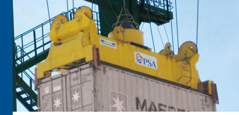
The RAM 3400 and 3500 series of All-Electric Telescopic Spreaders bring innovative standards of reliability, low maintenance and performance to container handling with the RAM 3400 series spreaders designed for ship-to-shore cranes and RAM 3500 for yard stacking cranes.
