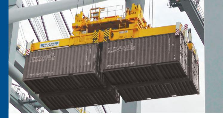
RAM's model 3350 is an innovative solution designed to allow single or multiple containers to be handled safely and reliably in a single crane operation to enhance container handling performance.
